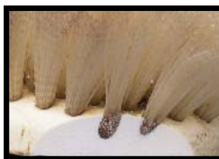
The staple-set brush illustrates that both filament and drilled hole area contain unwanted foreign matter that can be released during cleaning.
