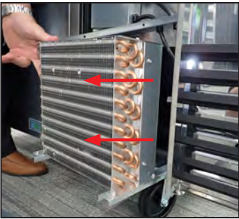
Fig. 6. Carefully slide the condensing unit out.
