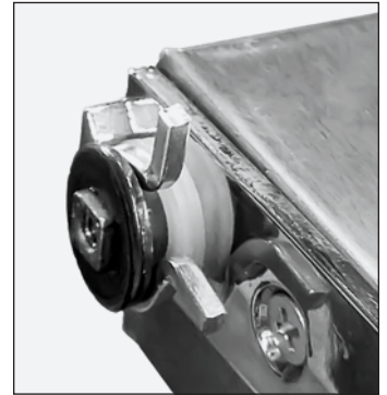
Fig. 7. Keep the washers in their original order.
