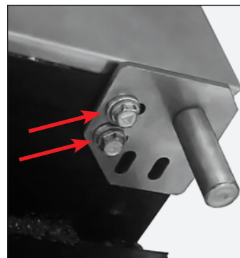
Fig. 9. Do not forget the washers.
