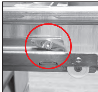
Fig. 5. Drawer retainer location. Retainer is engaged.
