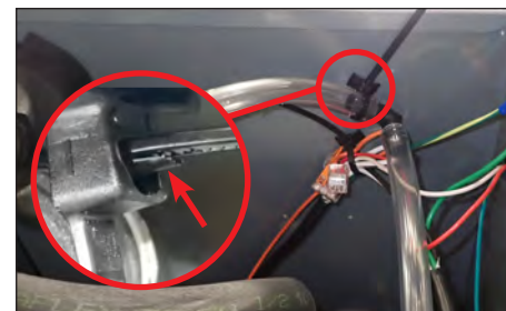
Fig. 3. Cable tie release tab location.
