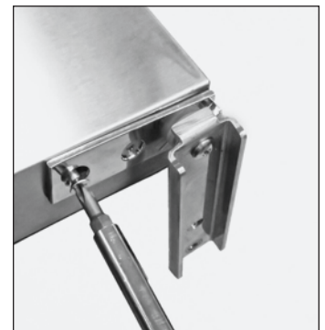
Fig. 5. Remove the cartridge hinge assembly.
