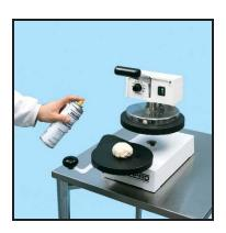
**STEP 1 -** After allowing upper platen to reach desired temperature, swing out lower platen and place pre-portioned ball of dough in approximate center and swing closed. An approved lubricant/release agent such as olive oil or DOUGHPRO's Cookware Food Release Spray # DPPC1 applied to the top of the dough ball will greatly improve the pressing operation.
