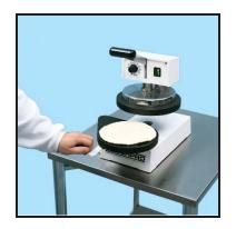
**STEP 3 -** Lift up handle, open platen and place flattened crust on screen, disc or pan. Now you're ready for make-up and baking.
