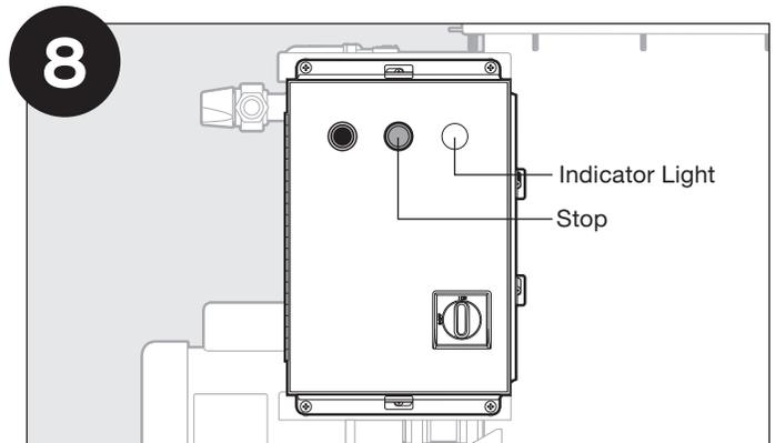
Press STOP on the control panel. Indicator light turns off.
