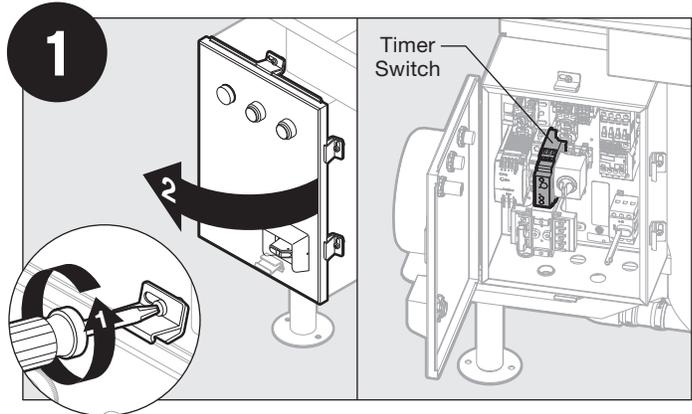
Open the control panel. Locate the Timer Switch.
