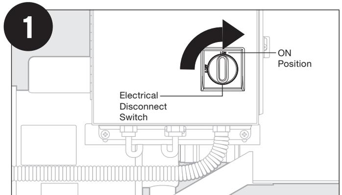
Turn electrical disconnect switch to the ON position. Open shutoff valves in water lines, if installed.
