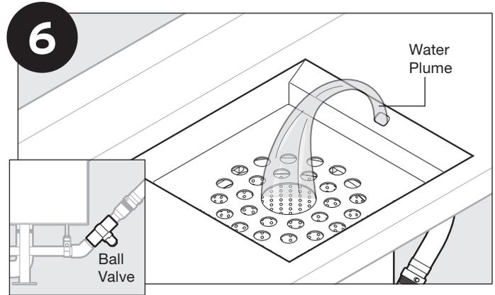
Adjust ball valve until water plume hits desired location inside tray area (recommended location is the center of scrap basket and/or cover).
