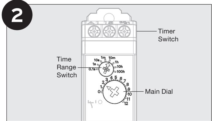
Rotate time range switch or main dial to desired settings (as shown). The time range switch sets the increments (0.1s, 1s, 10s, etc.) and the main dial is the "multiplier." The factory default is 10m on time range switch and 2 on the main dial, or 20 minutes.
