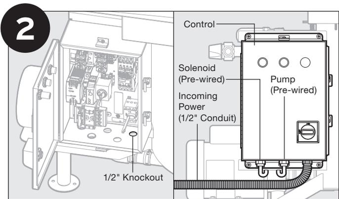
Run power from main power supply to the 1/2" knockout on bottom of control and connect as shown.
