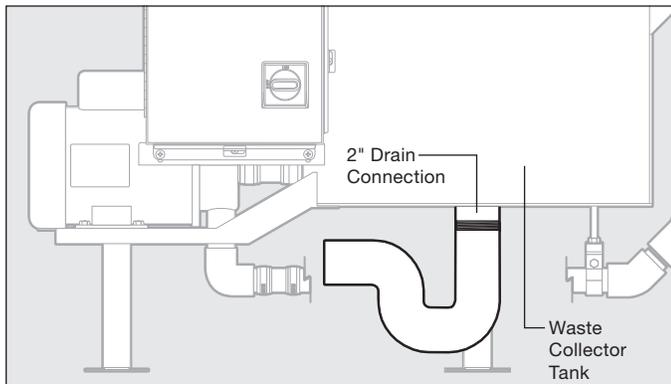
Figure 11. Drain Piping
