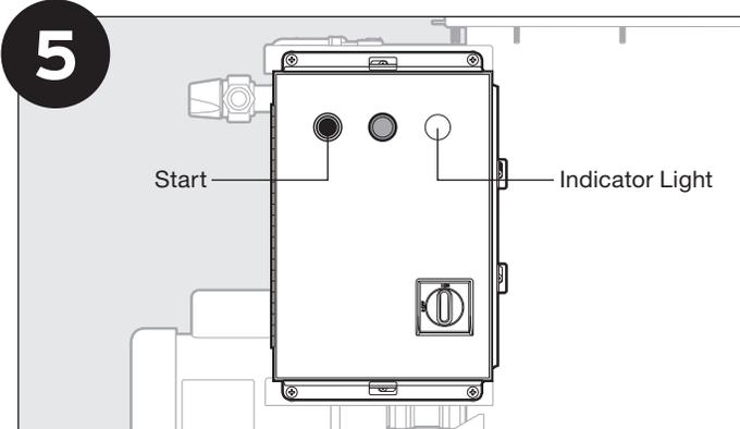
To begin, press START button on control and allow the reservoir tank to fill with water. Indicator light turns on. Pump turns on and water plume starts once tank has reached optimal fill level (approximately 70 seconds after pushing the START button).
