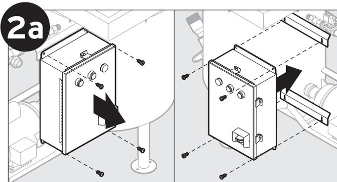
**Optional** – to relocate the control, remove and save four (4) bolts and nuts. Reposition box on other side of tank and secure with previously removed hardware. It is not necessary to disconnect factory-installed wiring.
