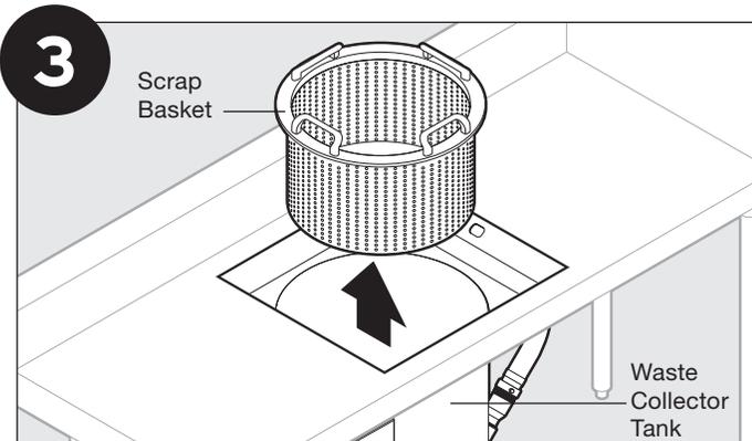
Remove scrap basket and dump waste into appropriate trash or compost receptacle.
