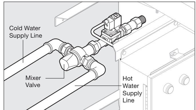
Figure 8. Water Connections
