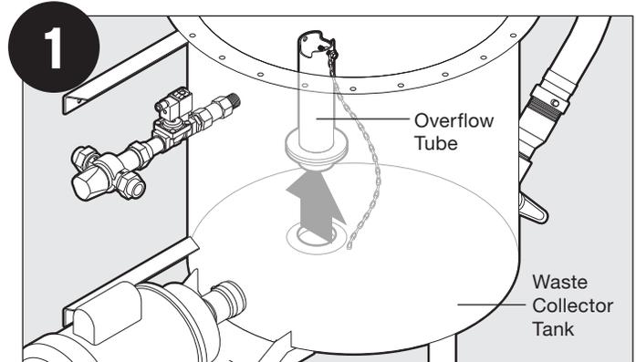
Turn off unit and empty scrap basket (see above instructions). Pull overflow tube to drain water inside waste collector tank.
