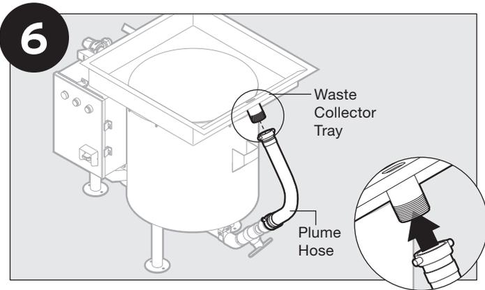
Connect plume hose to waste collector tray.
