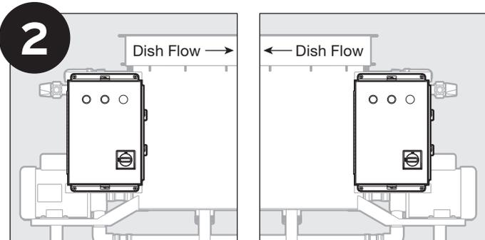
Verify dish flow and ensure that the control is on the proper side of the tank. The control should always face the operator and can be mounted on the opposite side of the tank if dish flow is reversed.
