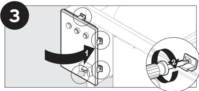
Close front panel and tighten screws on top cover retainers to secure.
