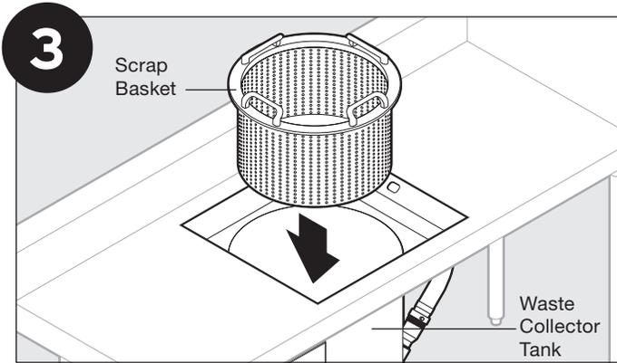
Place scrap basket inside waste collector tank. Unit must always have the scrap basket in place during operation.
