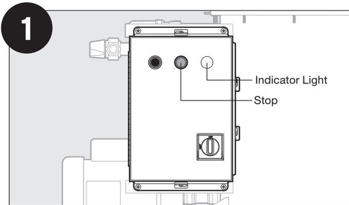
Ensure unit is turned off by pressing the STOP button on the control.
