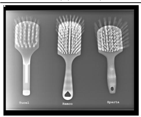
The above x-ray of three different utility scrub brushes illustrates the differences between Tucel's fused construction, whereby there is no metal elements holding filament to the block, whereas there are metal staples holding filament within drilled holes in the other two brushes. Holes harbor bacteria! (Remco and Sparta brushes purchased from Nelson/Jameson, Inc.)
