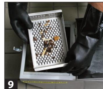
9 Carefully roll SDU from fryer; remove and empty crumb tray.
