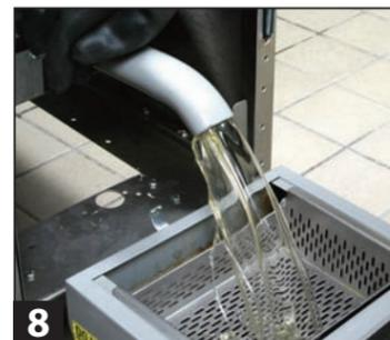
8 Open drain valve; drain oil into SDU; close drain valve. Remove and store drain extension.
