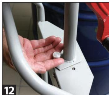
12 Release locking pin on pump head.
