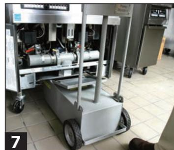
7 Slide SDU under filter drain down-spout.
