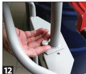
12 Release locking pin on pump head.
