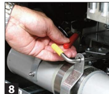
8 Open drain valve; drain oil into SDU; close drain valve.
