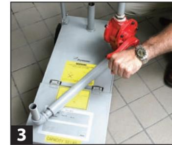
3 With the pump inverted turn the handle clockwise 3-4 turns stopping before oil pumps out of the spout.
