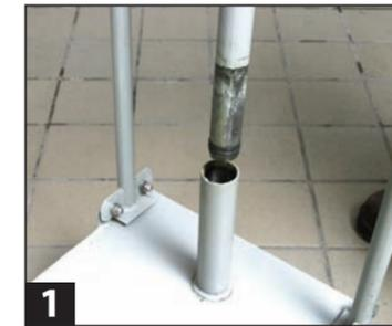
1 Remove the pump and pipe unit from the SDU by lifting up.
