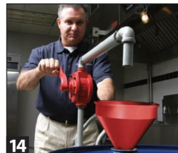
14 Attach hose or place funnel in oil disposal container opening. Turn pump handle toward spout to pump out oil\*.
