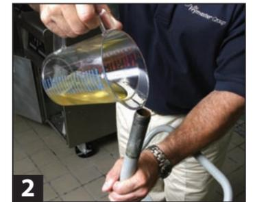
2 Invert pump and pour 1 cup of clean cooking oil into the pipe.
