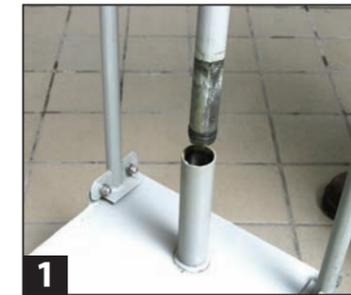
1 Remove the pump and pipe unit from the SDU by lifting up.
