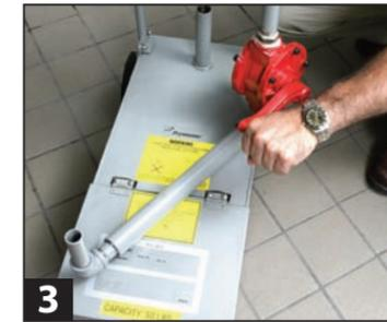
3 With the pump inverted turn the handle clockwise 3-4 turns stopping before oil pumps out of the spout.
