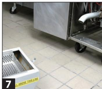
7 Position SDU under drain extension.
