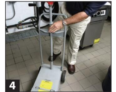
4 Reseat the pump and pipe unit on the SDU.
